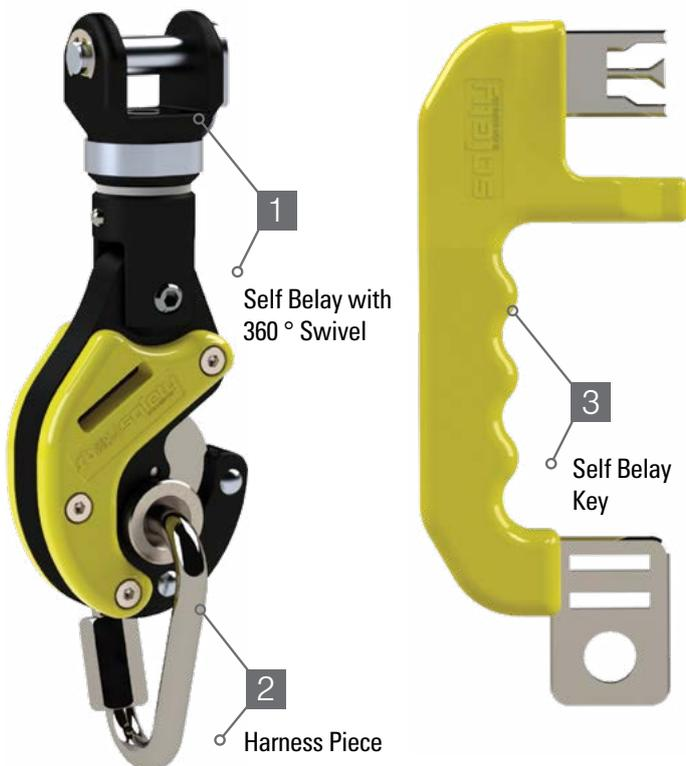
The Self Belay is an innovative climbing connector that increases the safety in climbing and adventure centers by only allowing users to climb when they are properly attached to the belay device.
